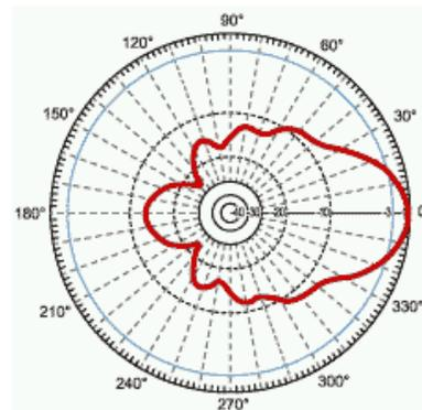
Fig. 6. Horizontal pattern for 14.5 dBi directional antenna
