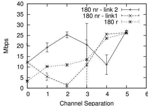
Fig. 3. Throughput results for routing vs. non-routing ( $180^\circ$ )
