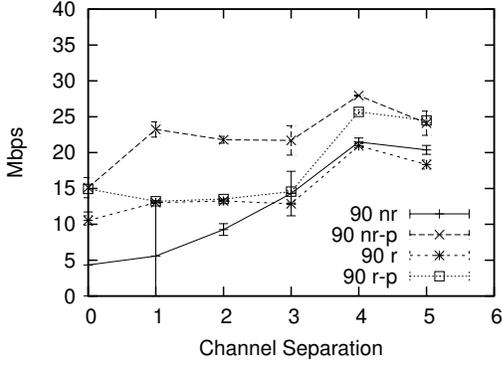
Fig. 7. Throughput results for mixed and uniform polarization on link 2
