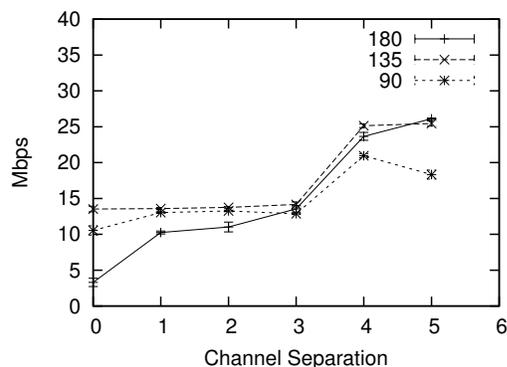
Fig. 4. Throughput results for the routing case with varying antenna separation (180°, 135°, 90°)
