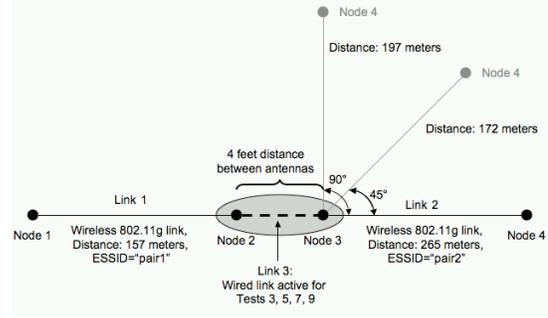
Fig. 1. Measurement setup
