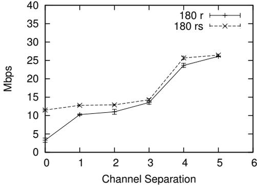
Fig. 8. Throughput results for additional separation in the vertical ( $180^\circ$  setup, 'r' routing without vertical separation, 'rs' routing and 4 ft vertical separation)
