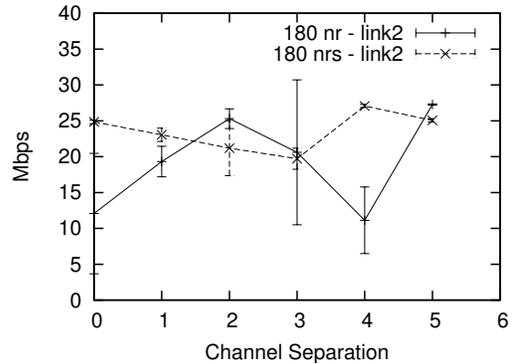
Fig. 10. Throughput results for link 2 with (nrs) and without (nr) additional separation in the vertical ( $180^\circ$  setup)
