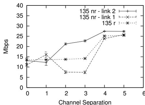
Fig. 5. Throughput results for routing and non-routing in the 135° case
