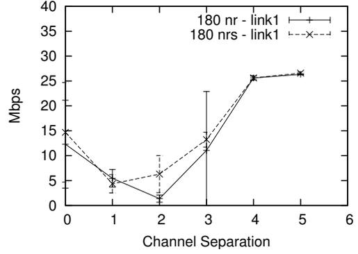
Fig. 9. Throughput results for link 1 with (nrs) and without (nr) additional separation in the vertical ( $180^\circ$  setup)
